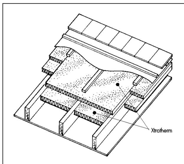
12.2 The board is light to handle but some handling difficulties may be experienced in windy conditions. Since the product will not support the weight of operatives, appropriate care must be taken during installation and tiling.
